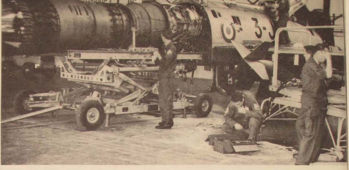
French Air Force mechanics make an engine change to keep their F-100 flying in the tactical exercise.
