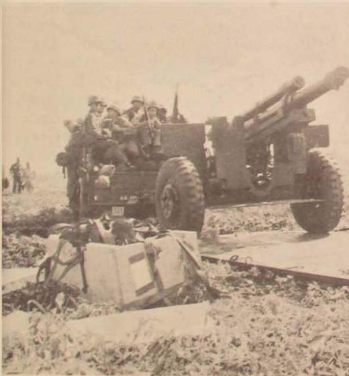
A gun crew of the 82d removes a 105-mm howitzer that was palletized and airdropped battle-ready.
